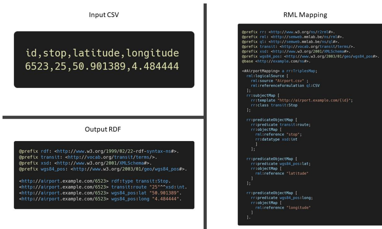
Figure 4.3: Example of an RML mapping from CSV to RDF
