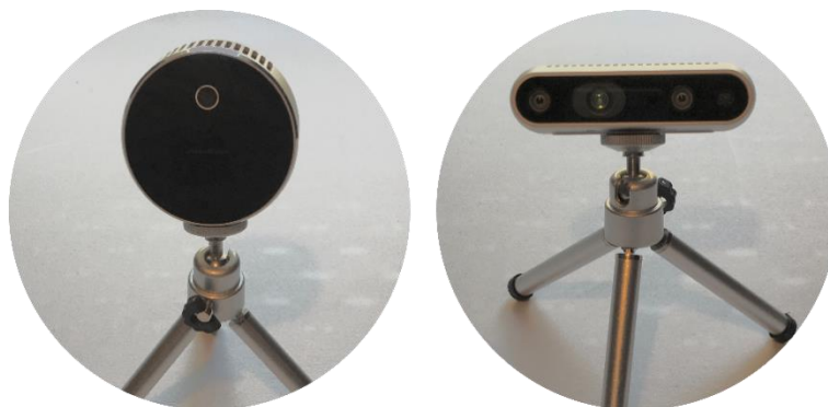
Figure 2-8. MEMS LiDAR cameras (left) and stereoscopic depth cameras (right)
