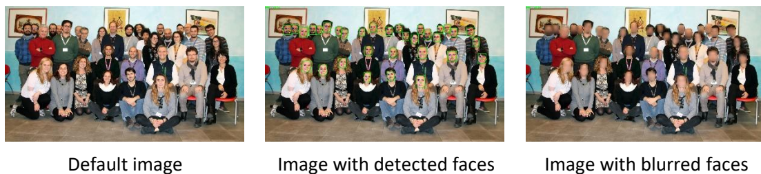
Figure 3-8: Sample results for the offloaded face blurring operation showing the original image (left), the image with faces detected by the algorithm (center), and the resulting blurred image (right).
